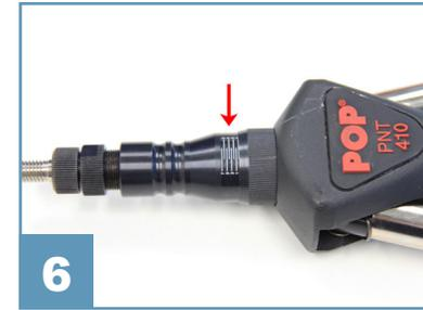
**6** Adjust the stroke of the mandrel at the head of the tool (up to M5 thread size start at 3mm; M6-M8 thread size start at 4mm; M10-M12 start at 5mm)
