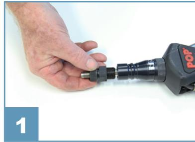
**1** To install the correct size mandrel and nosepiece in the tool, remove the nosepiece
