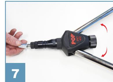
**7** Wind on the rivet nut with the levers fully extended.
