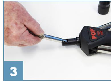
**3** Remove the mandrel by pushing and lifting. Replace with the correct size mandrel
