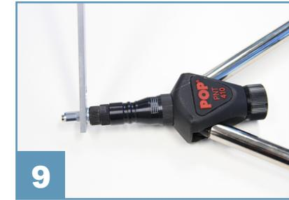
**9** Insert the rivet nut installed on the mandrel in the prepared hole. Bring the levers fully together in one motion
