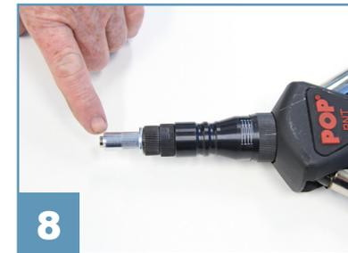
**8** Adjust the nosepiece so that the mandrel thread just protrudes through the end of the rivet nut
