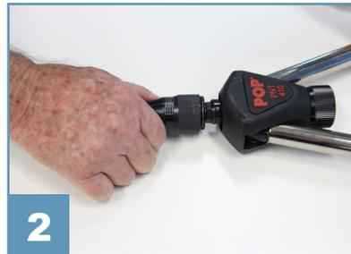
**2** Remove the front sleeve by pulling the sleeve from the tool
