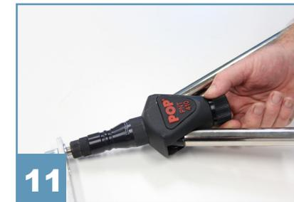
**11** Remove the mandrel for the rivet nut by rotating the mandrel holder knob anti-clockwise
